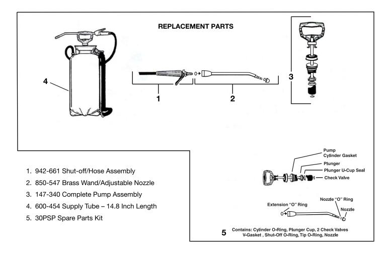
IMPORTANT: Replacement parts for No. 300P Sprayers made AFTER June 2018 are blue inked sprayer tanks. No. 300P Sprayers produced before June 2018 use black inked sprayer tanks and require different replacement parts – contact Nu-Calgon.
